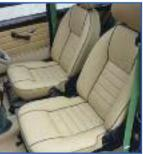
Primarily aimed at pre-1993 cars but suitable for all minis where the original seats have become worn or damaged beyond safe repair. Utilising a fully adjustable modern reclining mechanism and twin post, height adjustable head restraints, the seats also feature 6" (150mm) front to back travel on the seat slides. The subframe was designed to have the same floor footprint as a factory seat. The anti-tilt mechanism is a standard feature of the subframe.
