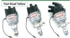
100AY A non-vacuum distributor, to suit most tuned engines, using camshafts such as Piper 270/285, Kent 266/276 and 286
