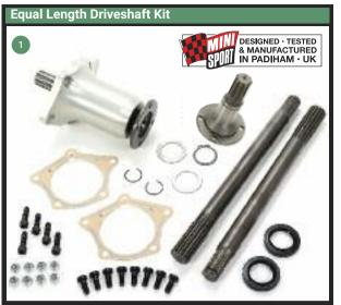
To reduce the effects of torque steer, equal length drive shafts are required. When the shafts are the same length torque steer can still occur, but only when the vehicles ride height is different on one side
