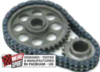
A lightened version of the Duplex timing set, designed especially for fast road and light competition. Reduces internal engine weight, therefore allowing the engine to rev faster.
