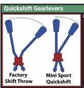
Improved feel, shorter gear lever travel and a faster, slicker gear change. Available for both rod type and remote type selector gearboxes, each kit comprises of a modified chrome gear lever, pivot retainer plus all mounting hardware. The Mini Sport Quickshift is easy installation job, which any reasonably competent enthusiast should be able to complete in a matter of 30 minutes.
