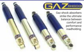
Easy 36 point rotary adjustment providing the facility for fine tuning without the need to remove the shock absorber from the car. Incorporates a double lip oil seal plus a further stem seal on the piston rod. Every unit is fully tested and dispatched from our factory with an individual report. Zinc plated body and accredited ISO9002 standard and supplied with a 2 year warranty.
