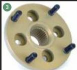
Sport product, created for competition Mini, where every gram of weight saving is critical. Losing 0.900kg over a standard Drive flange, giving exceptional weight loss from the un-sprung weight on the front of your Mini. Machined on our own CNC machines using 7075 aircraft specification aluminium billet, then hard anodised.
